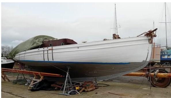
Spray in Dec 2024 showing undercoating
